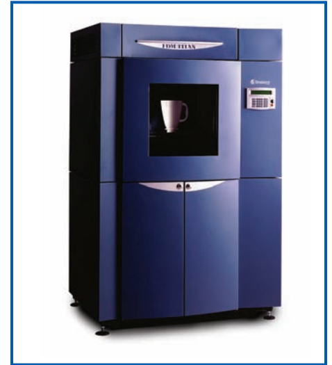
The Titan allows us to build functional prototypes with materials such as ABS.
