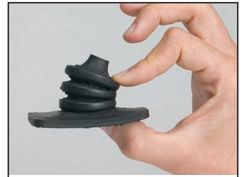
This soft SLA material has properties of 45 Shore A. This part was tinted black per customer request as a post cure operation.
