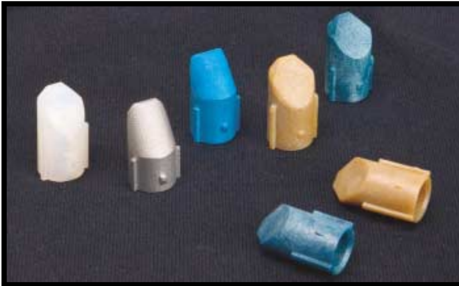
Using three rapid processes streamlined development of these small parts. From left: SL model, CNC-machined aluminum prototype, and injection-molded parts in various materials.
