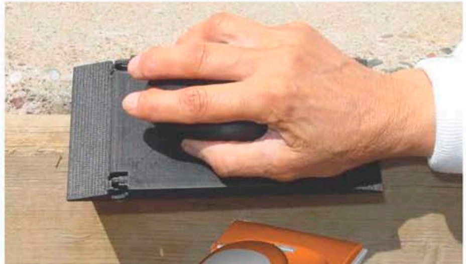
Top An FDM prototype of a new hand sander is used for functional testing before production tooling was released.
