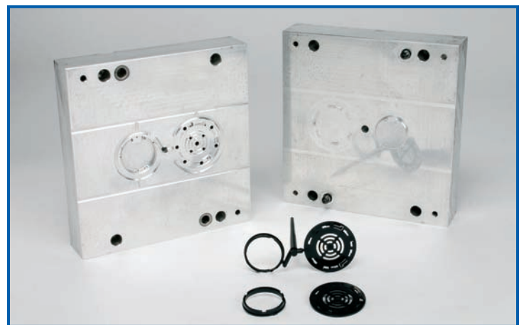
This 1+1 family tool shows different parts being shot at the same time. The runners, gates, and the center sprue are removed to complete the finished part.
