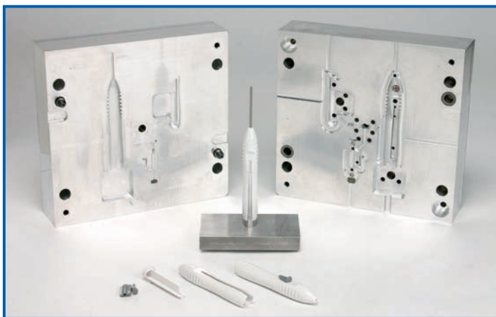
Above is a 1+1+1 family tool with a runner shut-off. Each part in this family tool has an undercut feature that has been captured with a hand pick-out.
